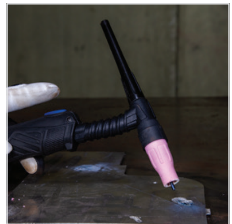
(3) Release the torch switch to bring in the end of the welding sequence dependant of 2T or 4T trigger function choice.
