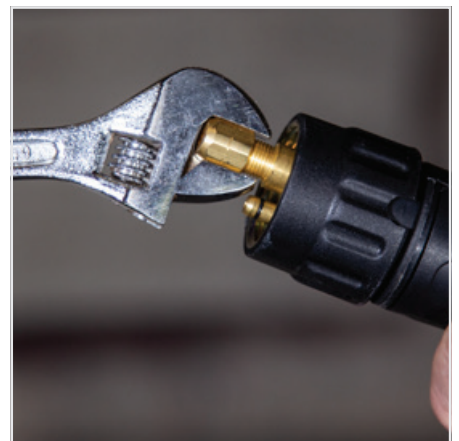
(9) Fully screw down the liner retaining nut and nip it up tight. This compresses the liner inside the torch cable assembly preventing it moving during use and ensures good wire feed.
