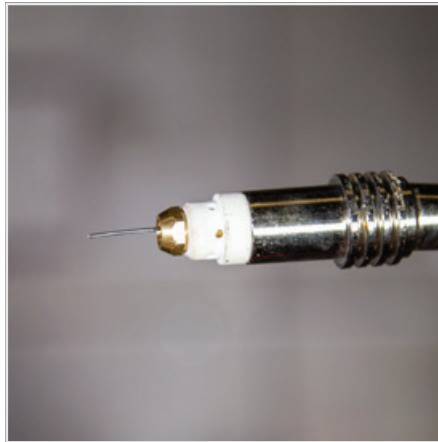
(10) Remove the gas nozzle and contact tip from the front end of the MIG torch.
