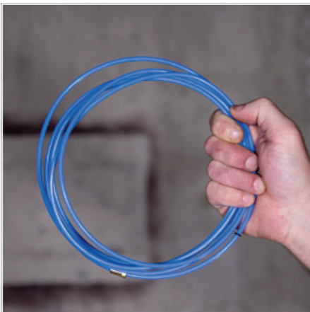
(4) Carefully unravel the new liner
