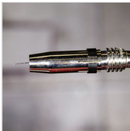
(17) Fit the remaining front end parts to the torch neck ready for welding.
