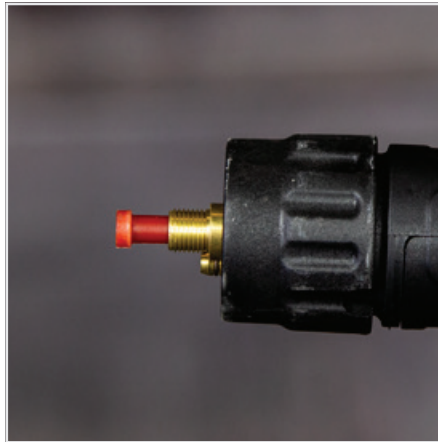
(2) Remove the liner retaining nut
