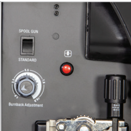
(12) Press and hold the inch wire button to feed the wire down the torch cable through to the torch head.
