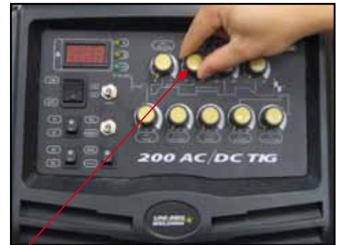
(11) Set the Peak Current (amps) to suit the tungsten size material type and thickness to be welded.
