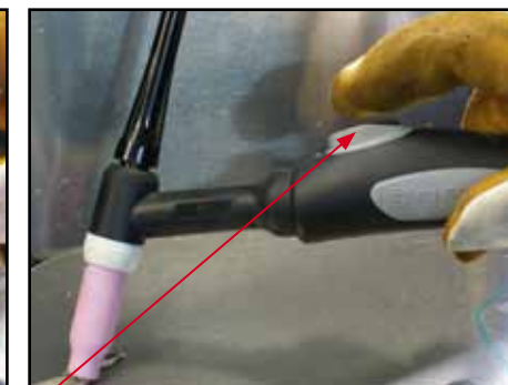
(6) Release the torch switch to bring in the end of the welding sequence dependant of 2T or 4T trigger function choice
