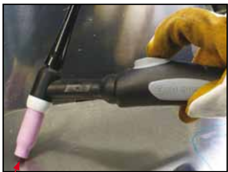
(4) Lay the outside edge of the Gas Cup on the work piece with the Tungsten Electrode 1- 3mm from the work piece
