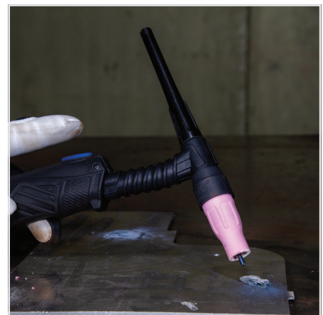
(3) Release the torch switch to bring in the end of the welding sequence dependant of 2T or 4T trigger function choice.
