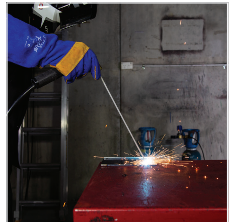
(5) Strike the electrode against the work-piece to create an arc and hold the electrode steady to maintain the arc.
