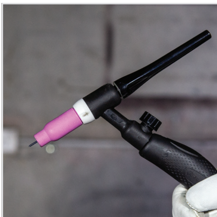
(5) Assemble front end parts of the TIG torch.
