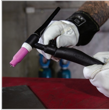
(2) Turn on the Gas Valve located on the TIG torch handle.
