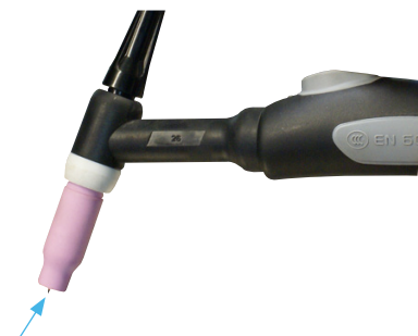
(1) Assemble the front end torch parts use the correct size and type of tungsten electrode for the job, the tungsten electrode requires a sharpened point for DC welding
