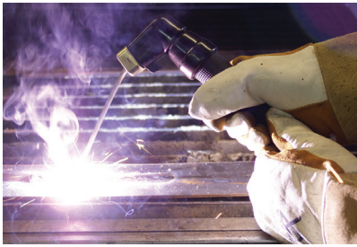
6) Hold the electrode slightly above the work maintaining the arc while travelling at an even speed.
