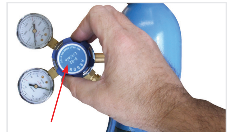
(14) Carefully open the valve of the gas cylinder, set the flow to 5-10 l/min
