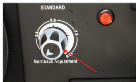
(16) Adjust the burn back control to prevent the wire sticking in the weld pool. Burn back control is located above the wire feed motor
