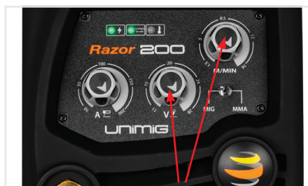
(16) Set welding parameters using the voltage and wire feed controls.
