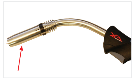
(14) Fit the gas nozzle to the torch head.
