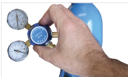
(15) Carefully open the valve of the gas cylinder, set the flow to 8-12 L/min
