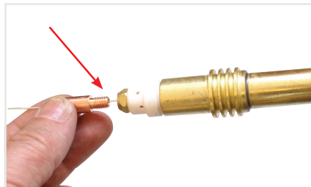
(13) Fit the contact tip over the wire and screw it into the tip holder, nip it up tight.
