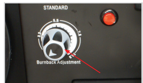
(17) Adjust the burn back control to prevent the wire sticking in the weld pool. Burn back control is located above the wire feed motor
