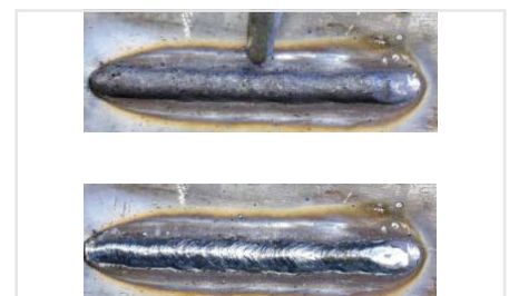
(8) Wait for the weld to cool and carefully chip away the slag to reveal the weld metal below.
