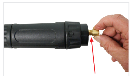
(6) Fit the liner retaining nut and screw only 1/2 way down
