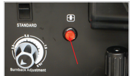
(11) Press and hold the inch wire button to feed the wire down the torch cable through to the torch head.
