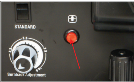
(12) Press and hold the inch wire button to feed the wire down the torch cable through to the torch head.
