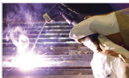
(6) Hold the electrode slightly above the work maintaining the arc while travelling at an even speed.
