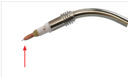
(12) Fit the correct size contact tip over the wire and fasten tightly into the tip holder.
