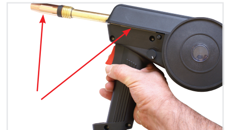
(14) Fit the gas nozzle and close the wire feed spool cover
