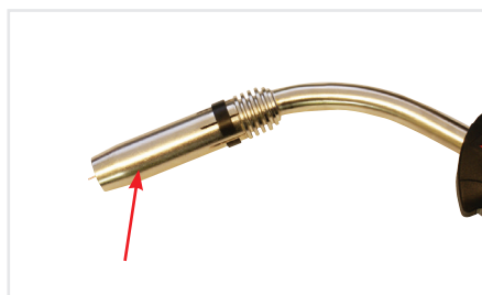
(17) Fit the remaining front end parts to the torch neck ready for welding.
