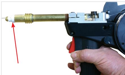
(12) Remove the gas nozzle and contact tip. Pull the trigger to drive the wire through the neck until it exits the contact tip holder
