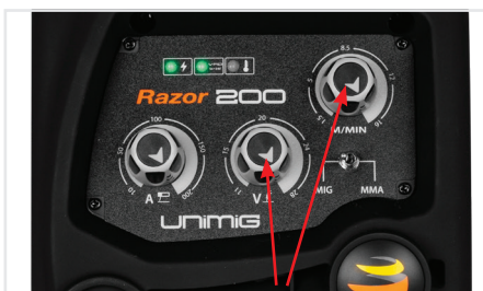
(15) Set welding parameters using the voltage and wire feed controls.
