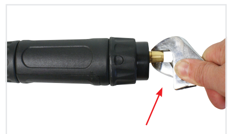
(9) Fully screw down the liner retaining nut and nip it up tight.
