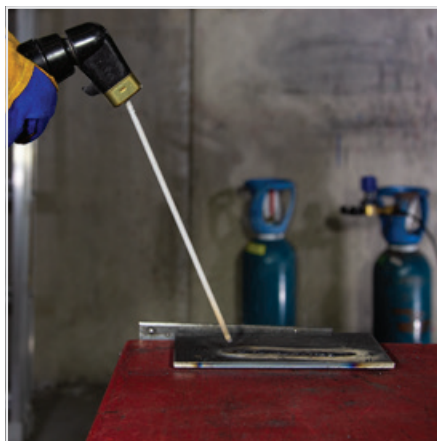
(7) To finish the weld, break the arc by quickly snapping the electrode away from the work piece.
