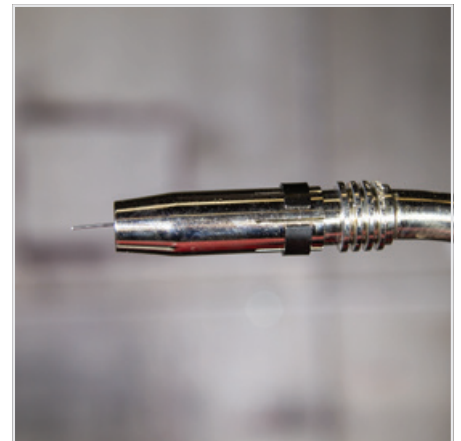
(14) Fit the gas nozzle to the torch head.
