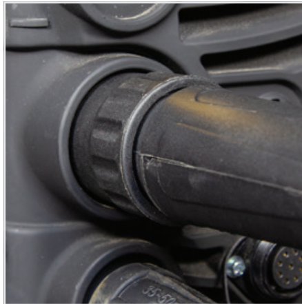
(14) Tighten and secure the torch Euro connector to the machine Euro receptacle
