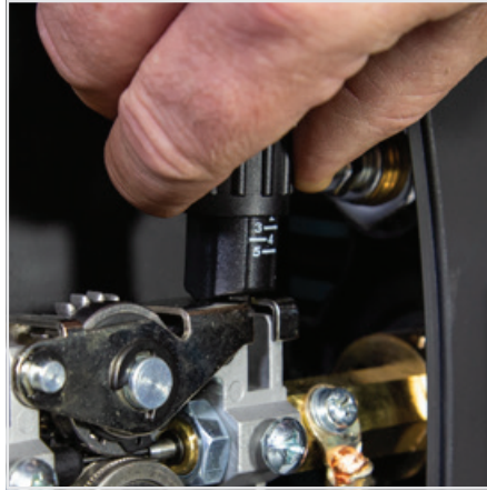
(10) Apply a medium amount of pressure to the drive roller.
