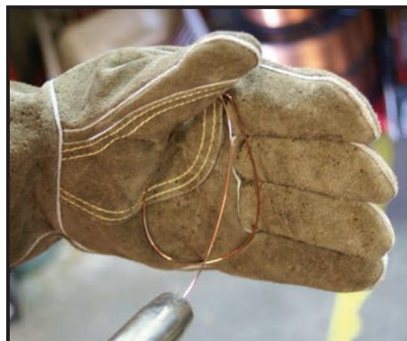
(8) A simple check for the correct drive tension is to bend the end of the wire over hold it about 100mm from your hand and let it run into your hand, it should coil round in your hand without stopping and slipping at the drive rollers, increase the tension if it slips.
