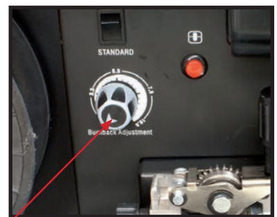
(17) Adjust the burn back control to prevent the wire sticking in the weld pool. Burn back control is located above the wire feed motor
