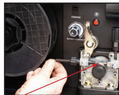
(12) Place aluminium wire onto spool holder. Feed the wire through and over the drive roller into the inlet guide tube.
