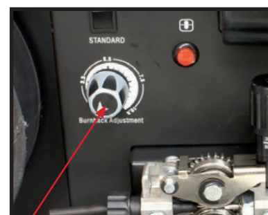
(16) Adjust the burn back control to prevent the wire sticking in the weld pool.
