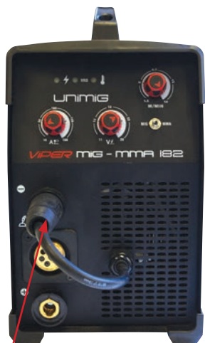
(2/5) Connect weld power lead to (-) negative terminal
