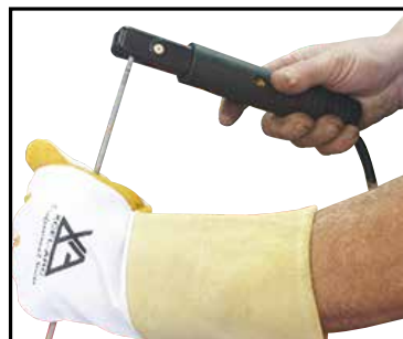
(4) Place the electrode into the electrode holder and clamp tight.
