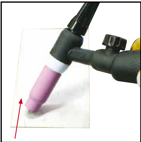
(9) Now drag the torch backwards lightly touch the tungsten to the work piece at the same time
