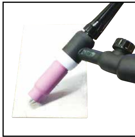
(8) Lay the outside edge of the Gas Cup on the work piece with the Tungsten Electrode 1- 2mm from the work piece.
